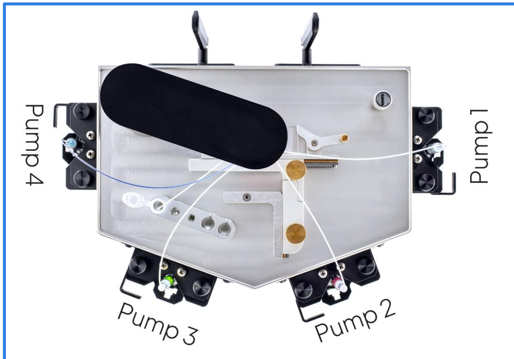
Figure 6. Microfluidic device connection diagram
