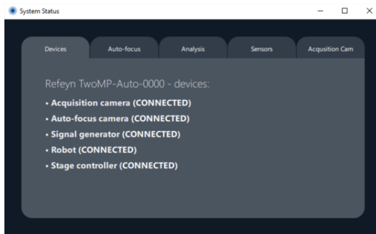
Figure 5: Dialog showing that all devices have started correctly, for Two MP Auto and Samux MP Auto. The dialogue for the One MP Auto will also list the DAC
