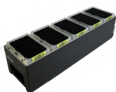
Tip Carrier TIP_CAR_480 containing five Tip Racks
