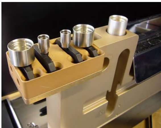
CO-RE Grippers mounted on waste block: 1000 µl Pipetting Channels (inner positions) and 5 ml Pipetting Channels (outer positions)
