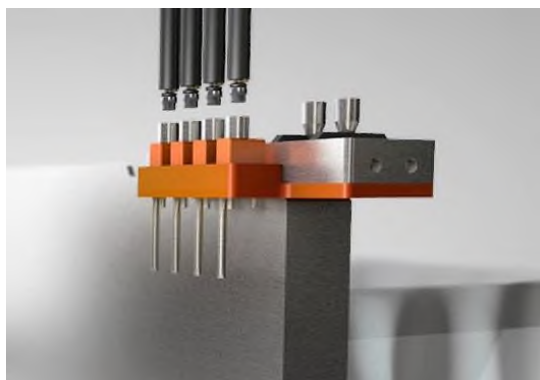
A Set of 4 FlipTube Tools (consisting of four fingers) within the holder
