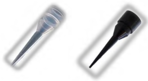
Clear and Conductive Low Volume CO-RE Tip, 0.5 µl – 10 µl
