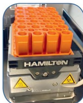
HHS 3 (PN 199085) equipped with a built-in adapter for a FlipTube Rack.
