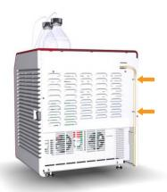
3 Cut the waste tubing to appropriate length. It is important that the tubing is not bent and will not be submerged in liquid during the run.
