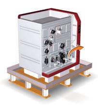
6 Prepare for lifting. Use two or more persons and grip the instrument from the front, from the back or from either side (only one side is shown below):
