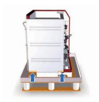
7 Lift the instrument over the foam attached to the plywood board, and pull away the board from under the instrument.
